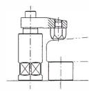
Swivel Contact Bolts are ideal for evenly distributing clamping pressure on sloped surfaces.
